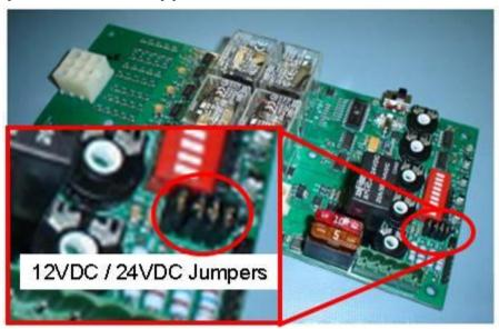
For 24VDC systems order the 24VDC board option (check model/serial number of transfer switch). If you have the 12VDC board option, remove the 5 jumpers to convert the board for 24VDC operation. Leaving the jumpers in will damage the board over time.
